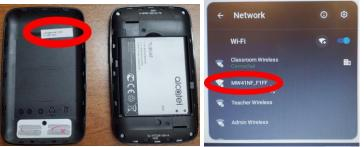
7. Enter the password that is listed on the small label located on the inside of the back cover of the hotspot.
